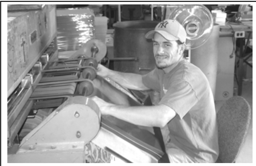
Chris Hall working on a slitter machine as he prepares the vinyl for Langstaff product line.
